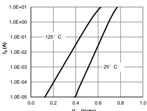
V<sub>SD</sub> (Volts) Figure 6: Body-Diode Characteristics (Note E)
