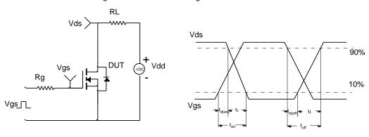
Figure C: Unclamped Inductive Switching (UIS) Test Circuit & Waveforms
