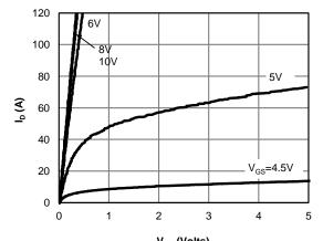
$V_{DS}$  (Volts) Figure 1: On-Region Characteristics (Note E)
