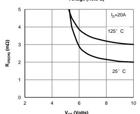
V<sub>GS</sub> (Volts) Figure 5: On-Resistance vs. Gate-Source Voltage (Note E)
