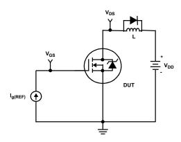
Figure 17. Gate Charge Test Circuit
