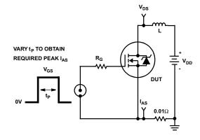
Figure 15. Unclamped Energy Test Circuit
