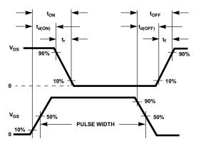
Figure 20. Switching Time Waveforms
