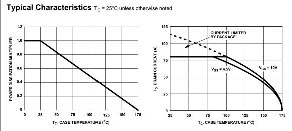
Figure 1. Normalized Power Dissipation vs Case Temperature
