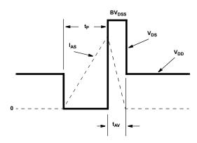
Figure 16. Unclamped Energy Waveforms
