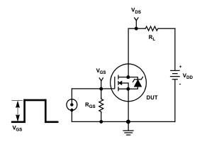
Figure 19. Switching Time Test Circuit
