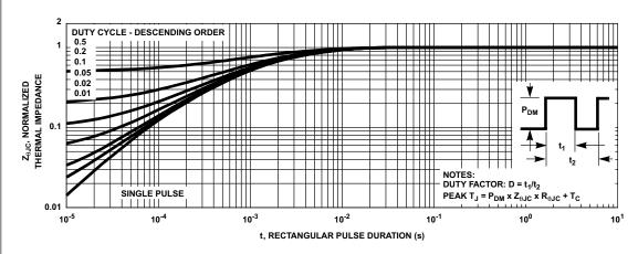
Figure 3. Normalized Maximum Transient Thermal Impedance
