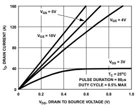
Figure 7. Transfer Characteristics
