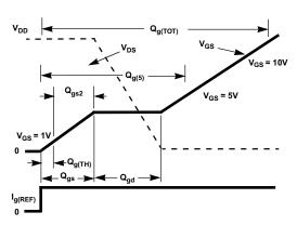
Figure 18. Gate Charge Waveforms
