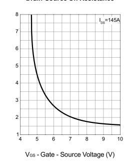
$R_{DS(ON)}$  - On - Resistance (m $\Omega$ )
