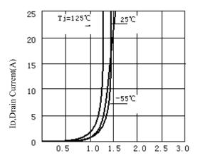
VGS, Gate-to-source Voltage (V) Figure 2. Transfer Characteristics
