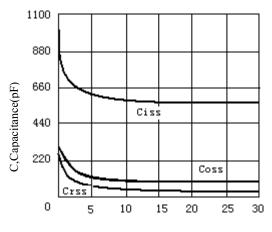
VGS, Drain-to Source Voltage Figure3. Capacitance
