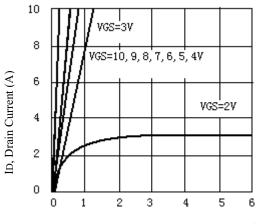
VDS, Drain-to-Source Voltage (V) Figure 1.Output Characteristics
