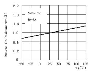
Figure 4. On-Resistance Variation with  $\label{eq:constraint} Temperature$
