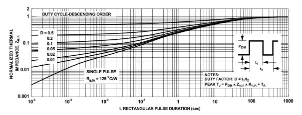
Figure 13. Junction-to-Ambient Transient Thermal Response Curve
