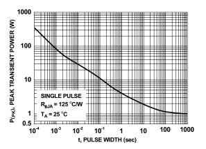
Figure 12. Single Pulse Maximum Power Dissipation
