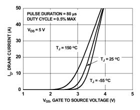
Figure 5. Transfer Characteristics
