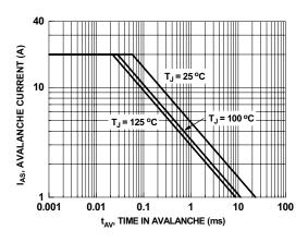
Figure 9. Unclamped Inductive Switching Capability
