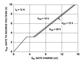
Figure 7. Gate Charge Characteristics
