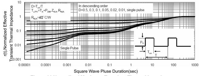
**Figure 11 Normalized Maximum Transient Thermal Impedance**
