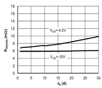
Figure 4 Drain-Source On-Resistance
