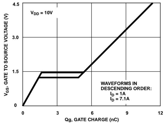
**Figure 13. Gate Charge Waveforms for Constant Gate Currents**
