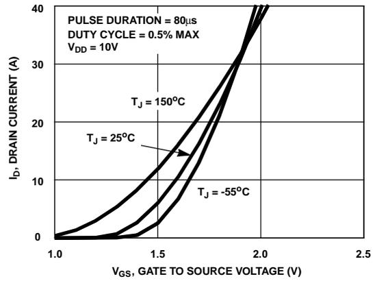
**Figure 6. Transfer Characteristics**
