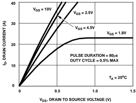
**Figure 7. Saturation Characteristics**
