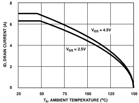
**Figure 2. Maximum Continuous Drain Current vs Ambient Temperature**
