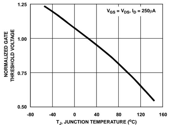
**Figure 10. Normalized Gate Threshold Voltage vs Junction Temperature**
