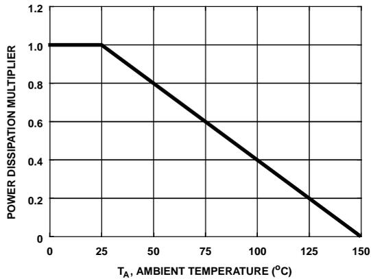
**Figure 1. Normalized Power Dissipation vs Ambient Temperature**
