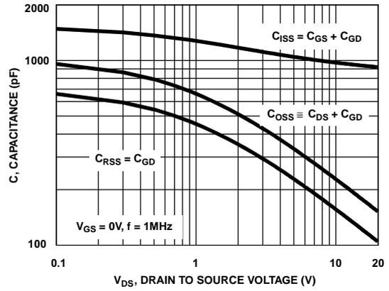
**Figure 12. Capacitance vs Drain to Source Voltage**
